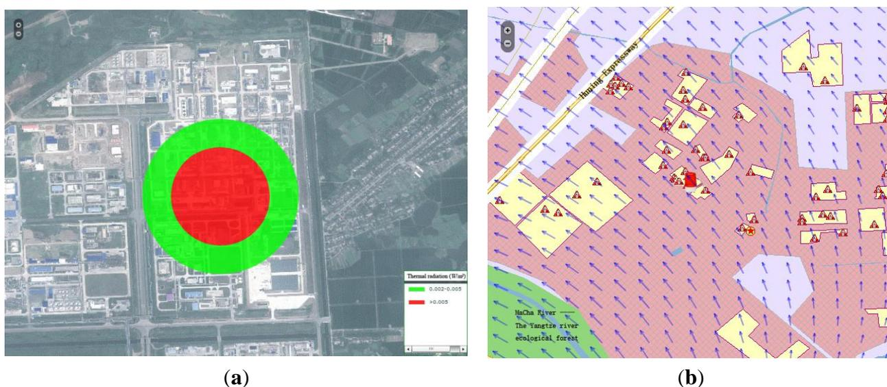
**Figure 4.** Time-series dynamic map for the leakage concentration field in the RS image (height 10 m). Images (a), (b), and (c) present the concentration field at the 5 min, 10 min, and 15 min, respectively, after the leakage accident.
